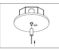
4. Screw the cable retainer to the stud from the mounting strap.
