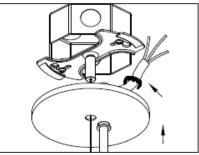
6. Remove the canopy. Install the bushing. Insert the cord end through the canopy. Then install the insulated crimp strain relief (hog ring) above the canopy. Bushing can be omitted if the cord is too large to fit through.
