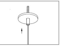
2A. If canopy is used, insert the canopy and securely fasten the cable retainer to complete installation.
