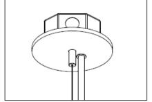
7. Install canopy to mounting strap. This completes the installation.
