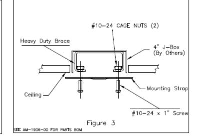
1. Insert the Heavy Duty Brace diagonally into the J-Box and align the holes to the bracket with the existing holes in the J-Box.
