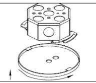
3. Temporarily install the canopy to the mounting strap
