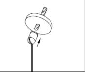
2A. If canopy is used, insert the canopy and securely fasten the cable retainer to complete
