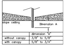
1. Secure the <sup>1</sup>/<sub>4</sub>-20 stud at the dimension shown. NOTE: Stud must be perpendicular to the slope ceiling.
